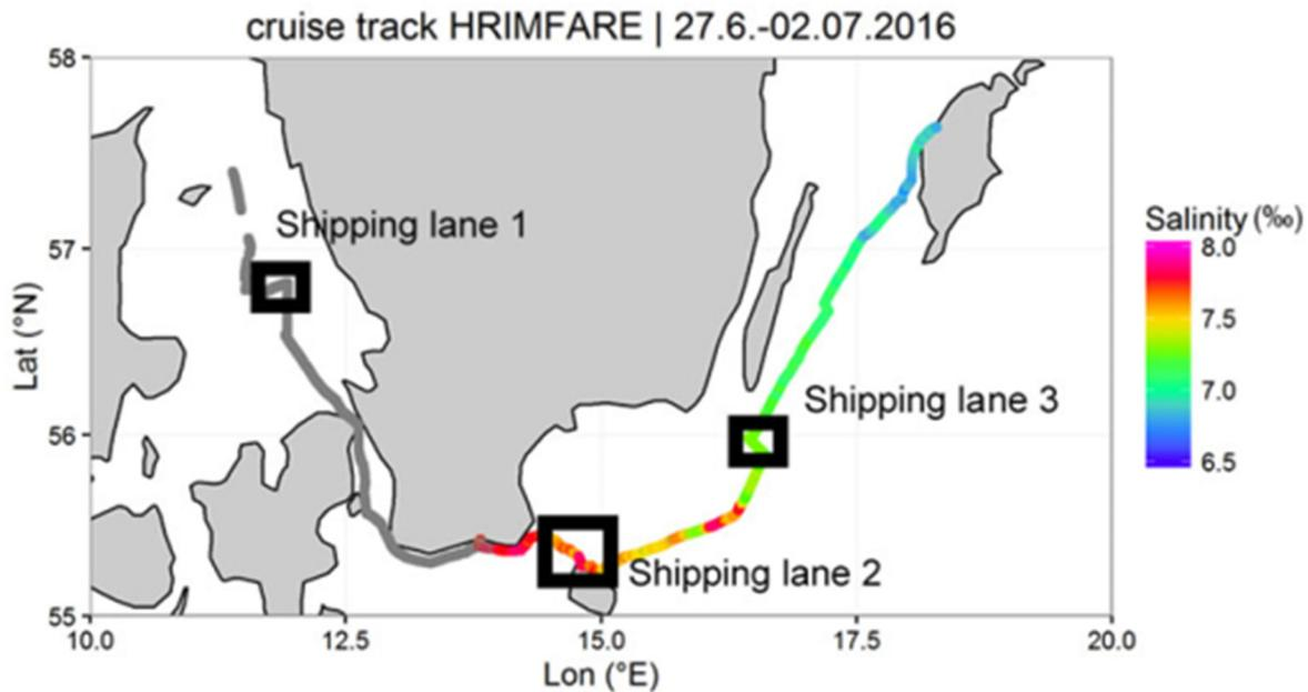
Figure 5: Cruise track of s/y Hrimfare and sampled areas in shipping lanes. Colored cruise track indicate the use of continuous measurement of salinity, temperature, pH, oxygen concentration and partial pressure of CO<sub>2</sub>. Grey cruise track indicate absence of such measurements. Courtesy of Martin Erikson, Chalmers.
