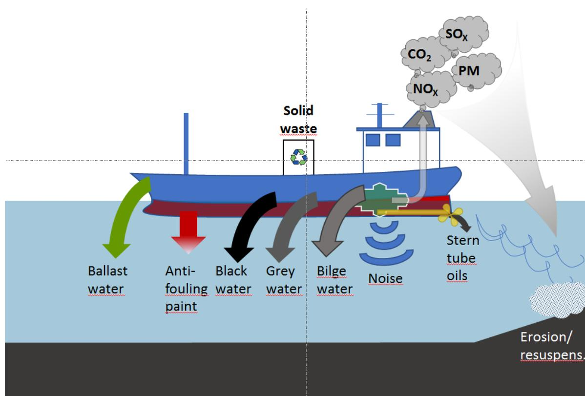
Figure 2: Sketch of discharges and emissions from ships into the marine environment. The terms black and grey water refer to sewage and wash water respectively. Bilge water originates from the engine room and is a mixture of condense water, oil, detergents and other cleaning agents (Figure prepared by Ida-Maja Hassellöv, Chalmers).
